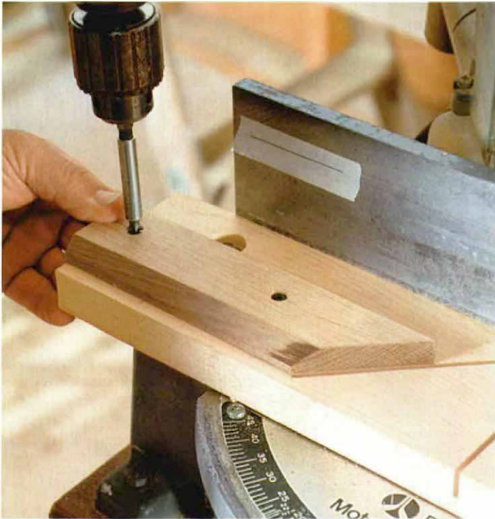
Miter-saw jig keeps correct spring angle. With the gauge block used to mark the crown height on the backing trim, the author transfers a mark to a piece of masking tape applied to the fence (photo top left). This mark corresponds to the mark on the wall measured by the gauge block. Holding a piece of molding upside down against the mark on the fence, the author transfers the molding's angle to the table (photo above). A length of scrap wood keeps the molding's angle proper (photo bottom left).
